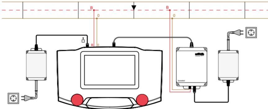
If you want to operate additional 60175 Boosters with the Central Station, then you can connect the 60125/60145 Terminal to the Central Station and connect up to four Boosters to each Terminal.
